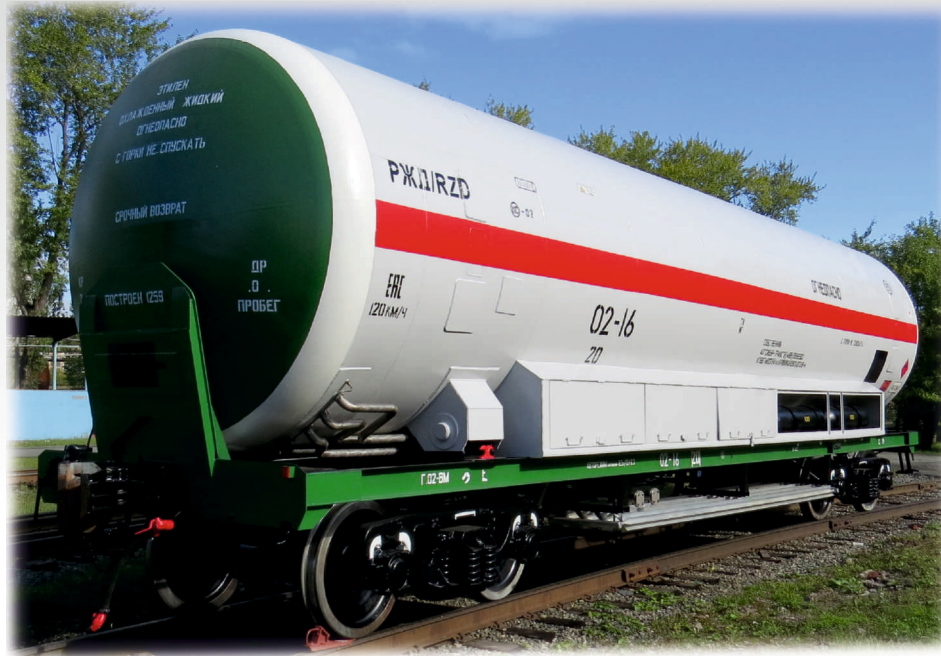
RAIL TANK CAR MODEL 15-5106 FOR TRANSPORTATION OF LIQUIFIED NATURAL GAS AND ETHYLENE
